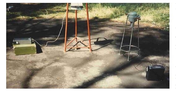
In situ measurement and sampling strategy defined in advance, and care taken to decontaminate according to measurement results. E.g., 'dripzones' near houses examined separately. Only the necessary soil layer was removed, thus minimising waste.
