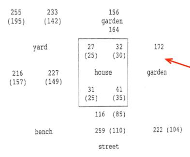
Removal depth was very inhomogeneous even over small areas and not optimised in relation to measurements of vertical distribution of contaminants. Russian army decontaminated 93 settlements in Bryansk Region in 1989: DRF = 1.1 - 1.5.
