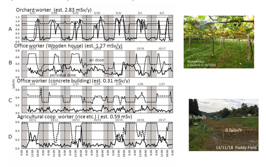
Spatial-temporal radiation exposure assessment using D-Shuttle with GPS/GIS technologies allowed for identification of peak exposure locations/times.
