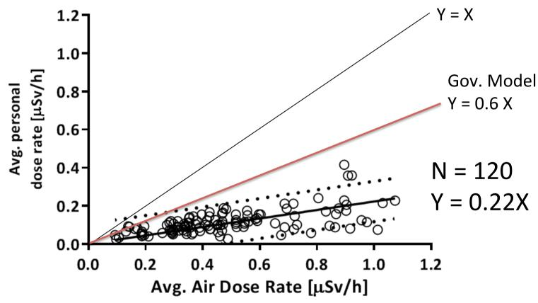
Additional personal doses obtained by D-shuttle were 22% on average of the corresponding cumulative air dose based on the airborne and car-borne monitoring surveys.
