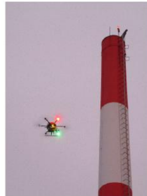
Figure 3: Illustration of UAV flight to collect radiation dose rates around the NRU stack.
