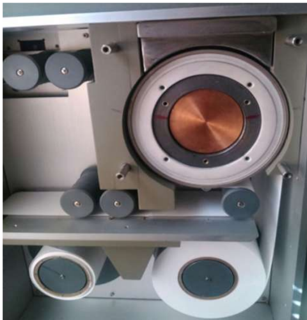
Continuous air monitor with in-situ HPGe-gamma spectrometer (CIEMAT)
