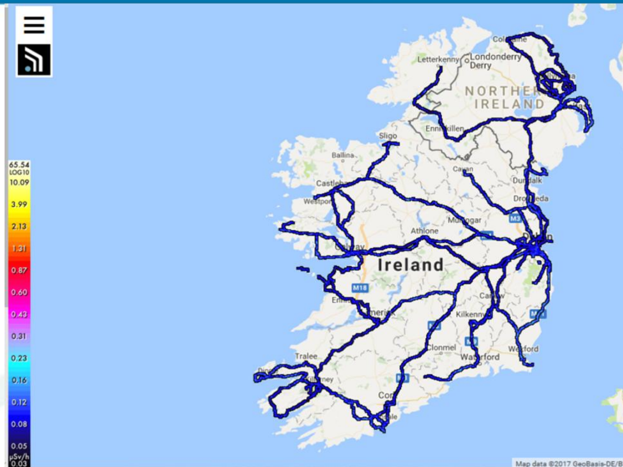
Figure 7: shows the Safecast API map of Ireland taken on the 25/04/18 which shows the measurements taken by the bGeigie Nano Monitor in blue around the country
