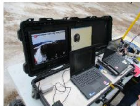
Figure 2: Portable ground station that communicates with the UAV.
