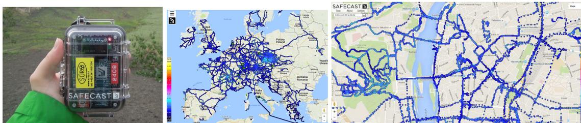
The Citizen Monitoring Network based on the above mentioned measuring devices and central application is designed, developed and implemented to enable transfer, storing, processing and presentation of measurement results together with their appropriate evaluation and explanation of their role in emergency preparedness and response.
