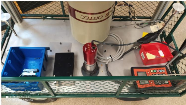
Detectors included in the in situ measurement and analysis gamma system.
