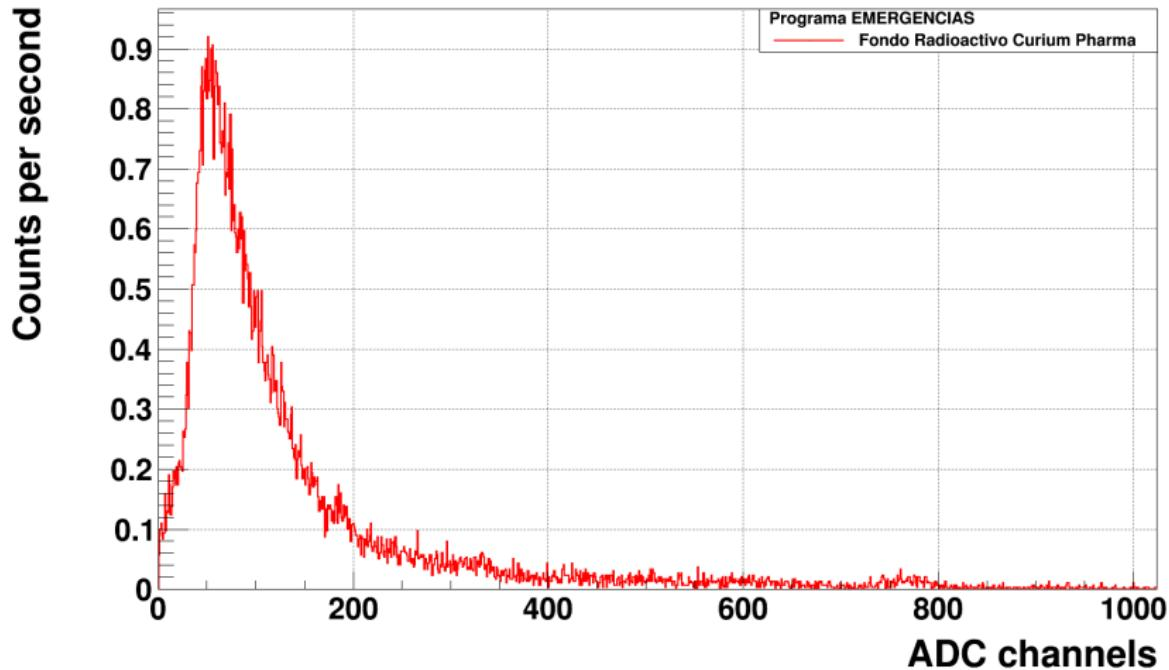
Energy spectrum measured at point 1 with the NaI detector.
