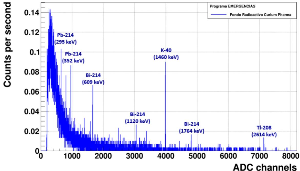
Energy spectrum measured at point 1 with the HPGe detector.
