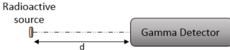
Experimental device used in the laboratory to calibrate and characterize the two gamma detectors.
