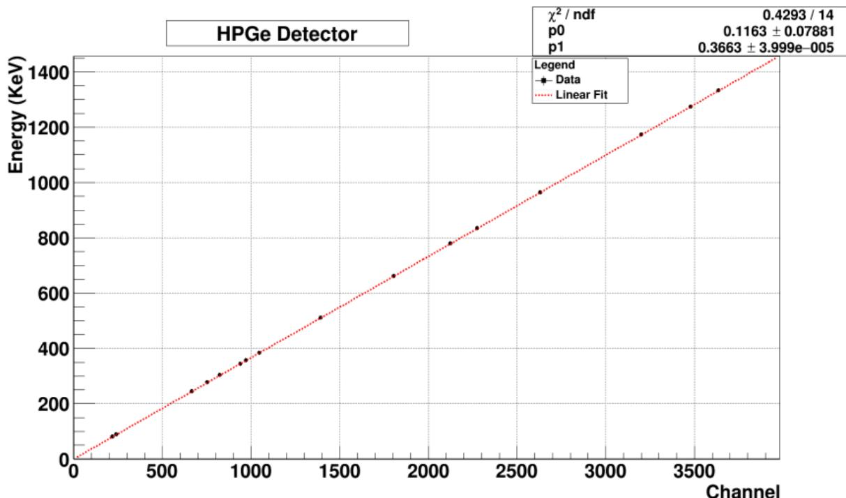
Linear fit for energy calibration of the HPGe detector.
