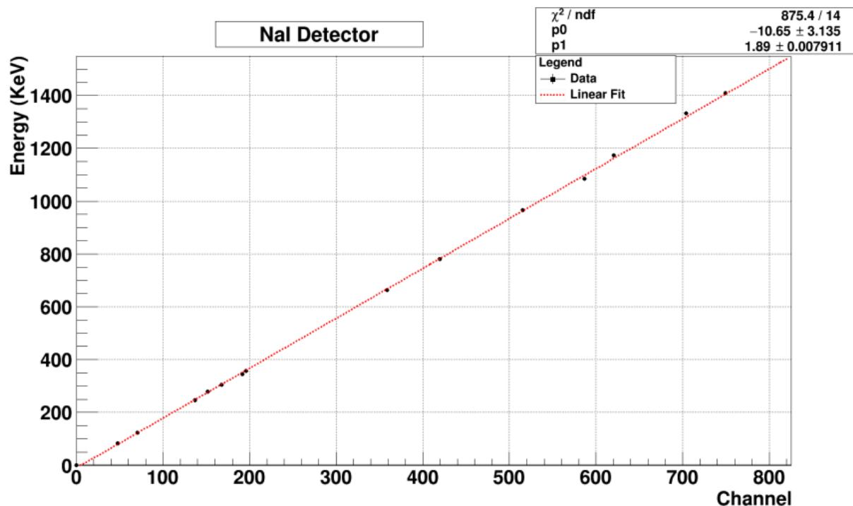
Linear fit for energy calibration of the Nal detector.
